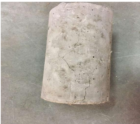
Fig 3: Cylinder specimen after testing
