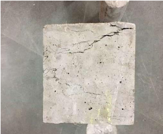
Fig 2: Cube specimen after testing
