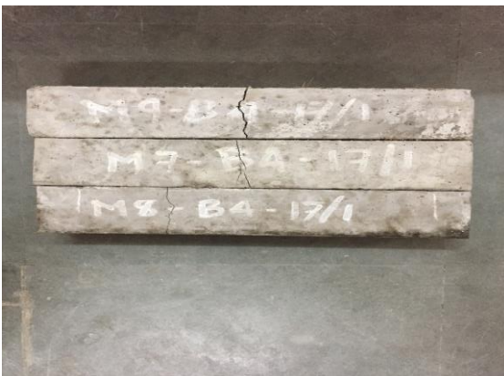
Fig 4: Beam specimen after testing
