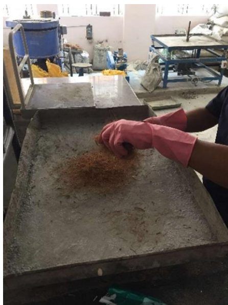
Fig 1: Weighing of Coir Fibre (10mm to 50mm in length)
