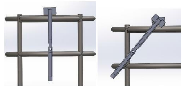
Fig -12: The concept of up and down rotation of the arm.
