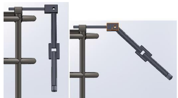
Fig-13: The concept of the sideways motion of the arm.
