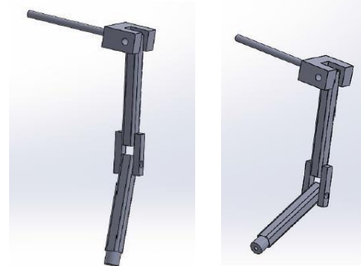
Fig-14: The concept of the up and down motion of the elbow
