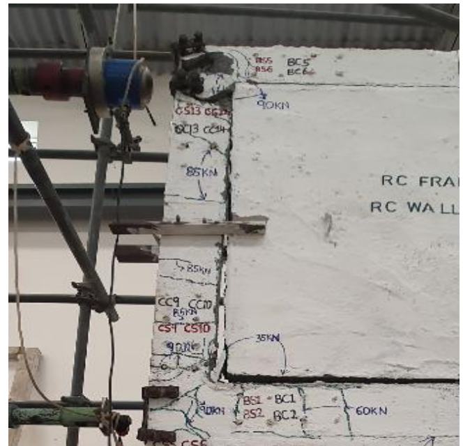
Fig -14: Top storey cover crushing
