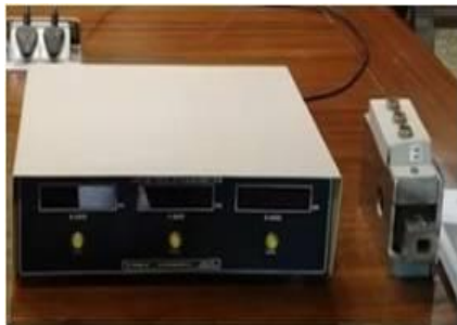
Fig-6 CNC Lathe dynamometer setup
