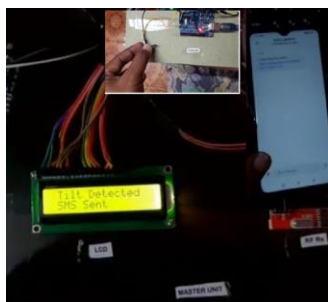
Figure 17: When tilt Detected by Accelerometer Sensor then SMS send to registered number
