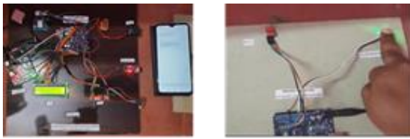
Figure 14: When Pulse Rate Detected by Pulse Rate Sensor then SMS sends to Registered number
