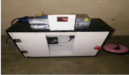
Fig 10. Refrigeration body after fabrication
