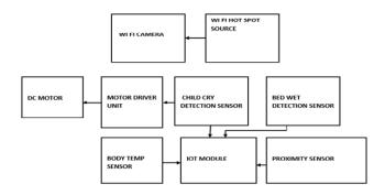
Block diagram of prototype model is as shown in the figure which represents all the units of the proposed system. Sound sensor continuously hears the frequency, when infant starts to cry cradle will start swinging. Also, parent will be intimated by message alert through the IOT module if the
