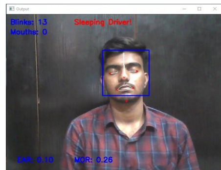
Snap 4: Drowsiness detected due to sleep, EAR value is very low, and hence alarm is raised.
