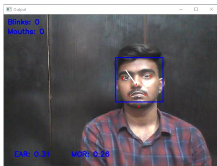
Snap 1: This is normal/Ideal condition where the face of person is detected with the specified features, EAR (0.31) is greater than the threshold value (0.28) and MOR (0.26) is less than threshold value (0.3) hence no alarm.
