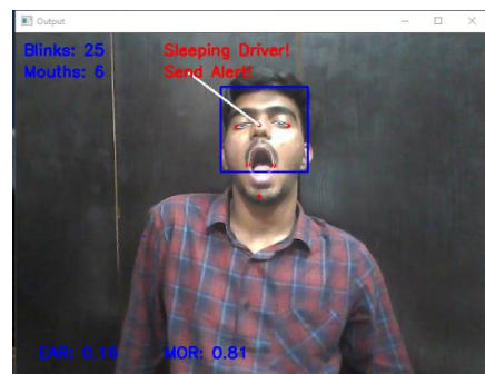
Snap 5: Due is high decrease in EAR value and high increase in MOR value, alert is sent and alarm is raised.
