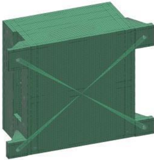
Fig. 5. Boundary Conditions for Modal and Static analysis
