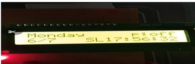
The microcontroller gets the current date and time from DS1307 RTC and to turn on a relay that supplies 5 volts to the pump. LCD display information about the different conditions of the soil and shows the real time and date using RTC component. When the desired moisture level is reached, The relay will off. Then microcontroller will send signal to the motor. This will result in turning off the motor.
