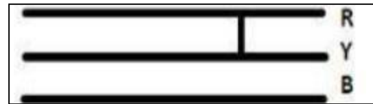
Fig. 2: Line to Line Fault
