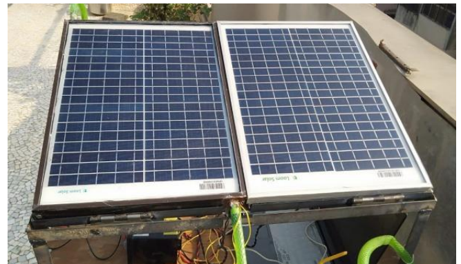
Fig 5 – PVT module and PV Panel
