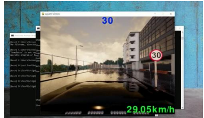
Fig 2: Sign Board Detected by passing each frame through Yolo module to Detect Speed Sign
