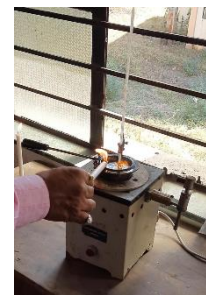
Fig -9: Flash and fire point
