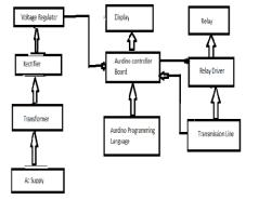
Fig:-1 Block Diagram
