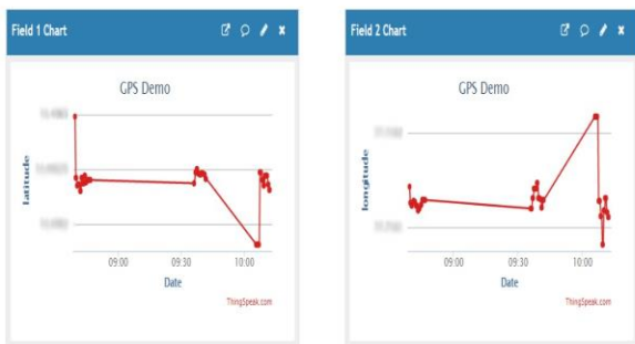
Fig-2: The latitude and longitude values obtained from the Neo 6M GPS Module and plotted by ThingSpeak
