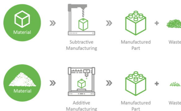
Fig-1 : Concept of Additive Technique
