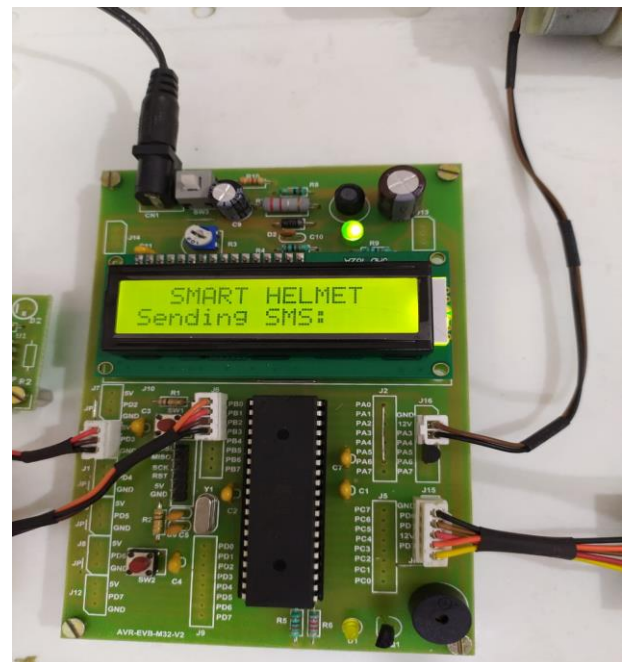
Fig 16: Emergency Message Display
