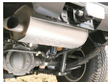
Fig -2: Leaf spring on vehicle [2]
