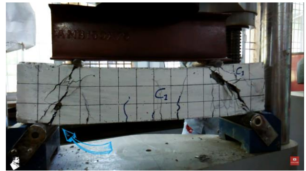
Fig -2: Failure of RCC beam
