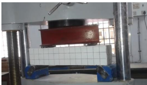
Fig -1: Testing on RCC beam
