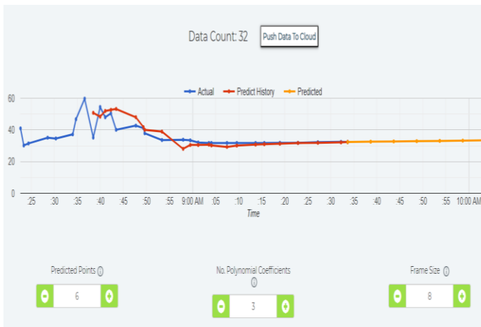
Fig.11 Output for the predicted temperatures and a comparative analysis of actual and predicted.
