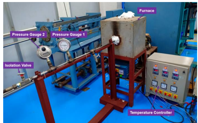
Fig -5: Thermal Cycling Test setup
