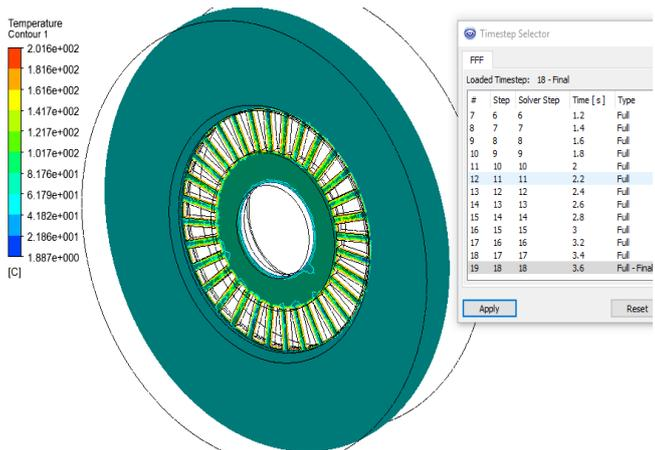
**Fig -26:** Shows temperature of disc, case 3 at 3.6 sec
