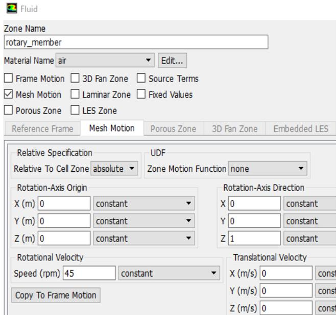
Fig -16: Shows the rotary boundary conditions
