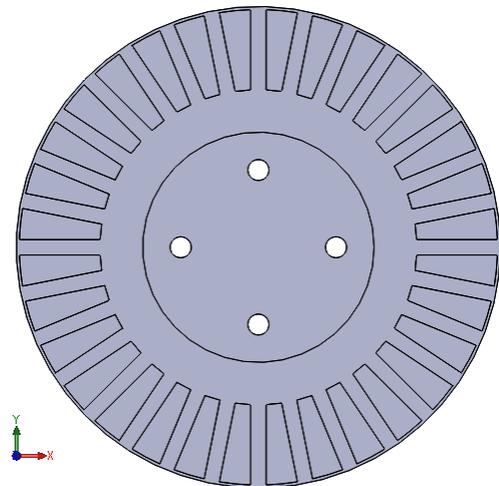
Fig -5: Shows the 3 D model of the disc for case3 for CFD analysis
