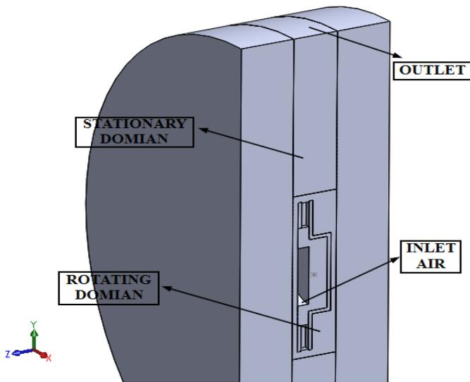
Fig -12: Shows the description of CFD model
