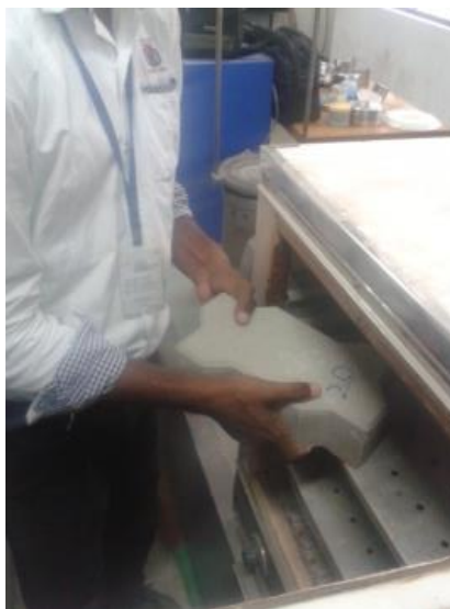
Fig -2: Water absorption test
