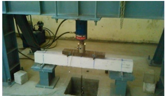
Fig-5 Loading Frame Setup
