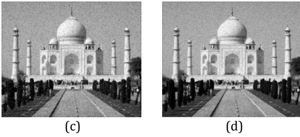
Fig-19: Noise removal process carried out by Average/Mean filter over images with (a) Gaussian noise (b)Poisson noise (c)Salt & Pepper noise and (d) Speckle noise
