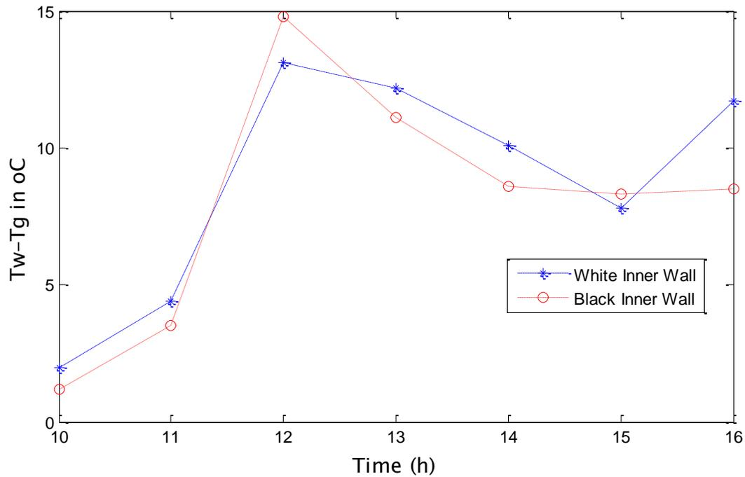
Fig 3 Difference between Water Temperature and Glass Temperature ( $T_w-T_g$ ) with respect to time for Black Inner Wall and White inner wall solar still for a typical day of month May-June 2014
