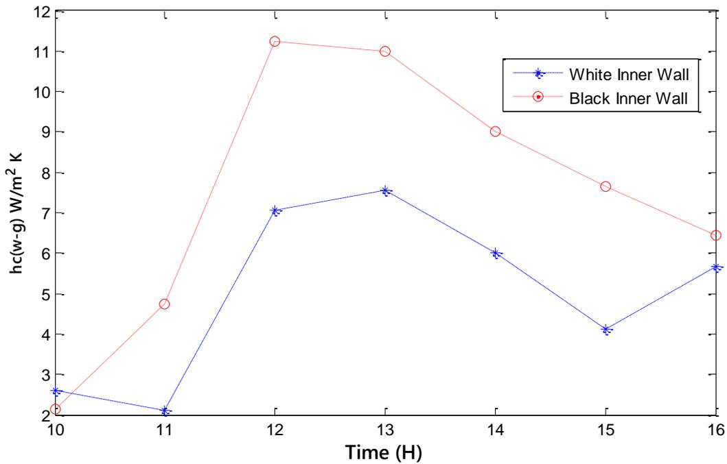
Fig. 5 variation of convective heat transfer coefficient between water and glass with respect to time for white and black inner wall
