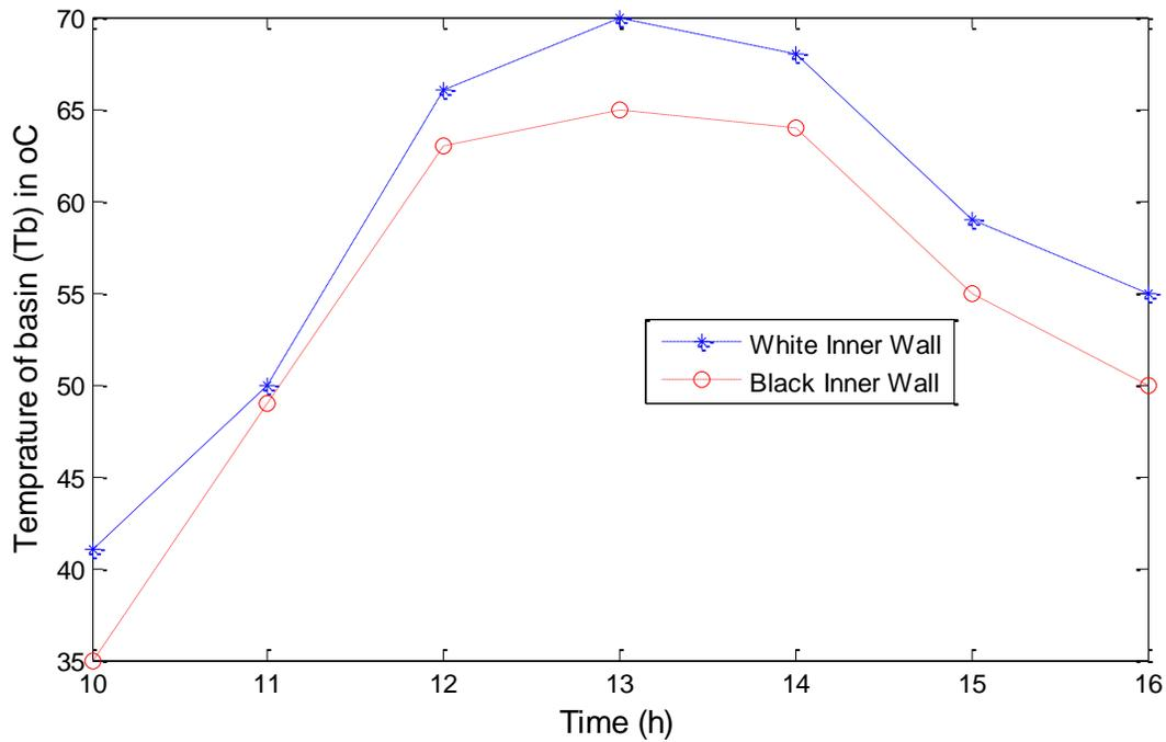
Fig 1 Hourly Variation Of Temperature of basin for Black Inner Wall and White inner wall solar still for a typical day of month May-June 2014
