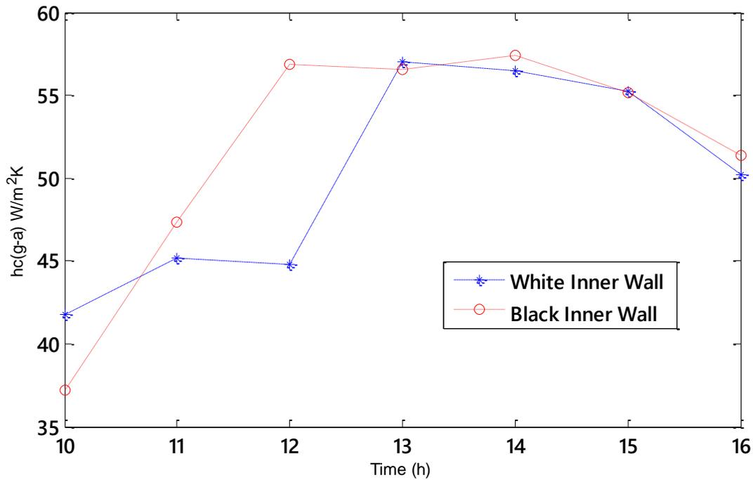
Fig 7 variation of convective heat transfer coefficient between water and air with respect to time for white and black inner wall
