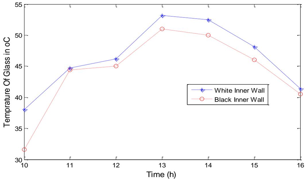
Fig 2 Hourly Variation of Temperature of Glass for Black Inner Wall and White inner wall solar still for a typical day of month May-June 2014
