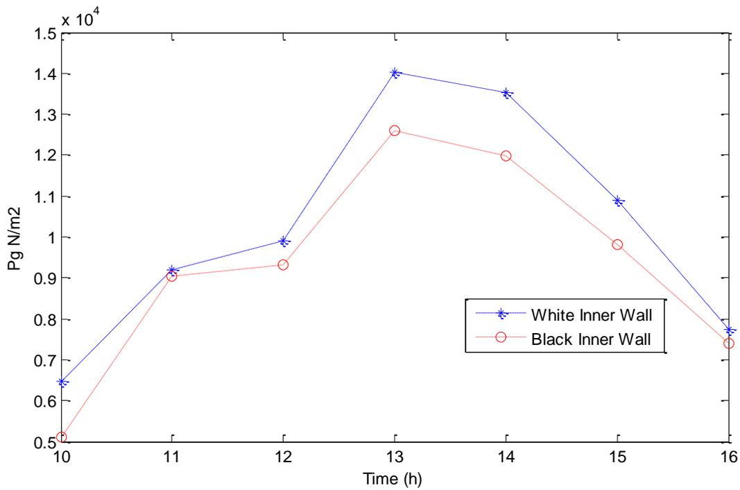
Fig 9 Variation of pressure at glass surface with respect to time for white and black inner wall
