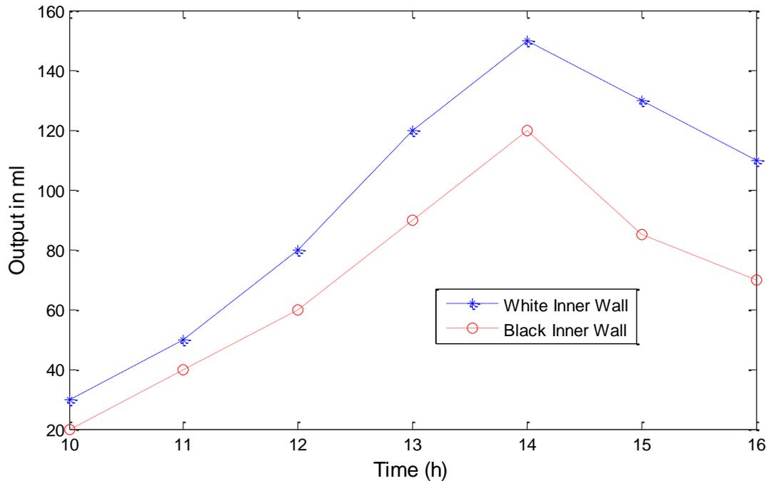
Fig 4 Fig Hourly Variation Of Output of Black Inner Wall and White inner wall solar still for a typical day of month May-June 2014
