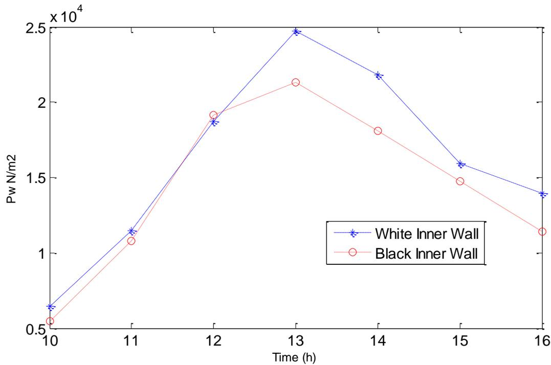
Fig 8 Variation of pressure at water surface with respect to time for white and black inner wall
