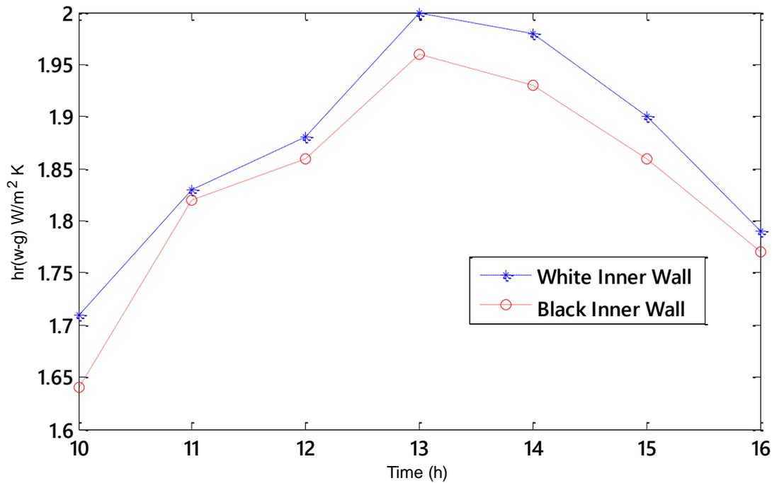
Fig. 6 variation of radiative heat transfer coefficient between water and glass with respect to time for white and black inner wall
