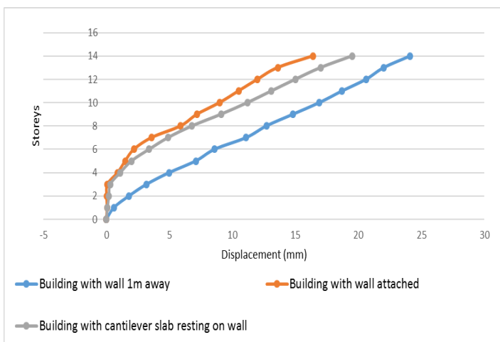
Fig. 9: Displacement of buildings for time history analysis
