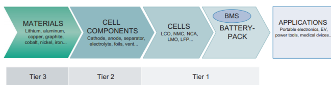
Fig 3.[9] Manufacturing stages of LIB
