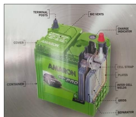
Figure1. Structure of lead Acid Battery
