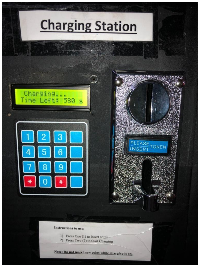
Fig - 12: Displaying “Charging Started and Time Left”.
