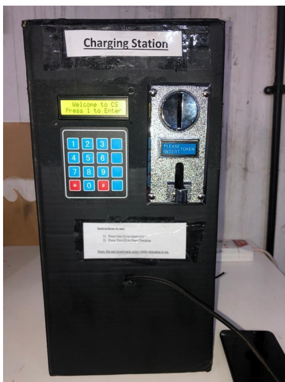
Fig - 9: Implemented Mobile Charging Station.
