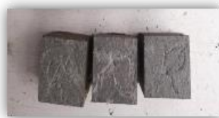
FIG 2 CASTING OF CUBES
