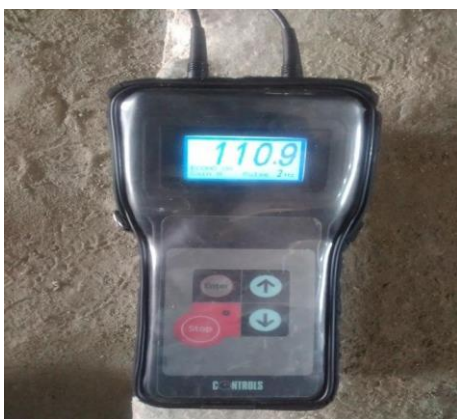
Picture 2- Ultrasonic pulse velocity device
