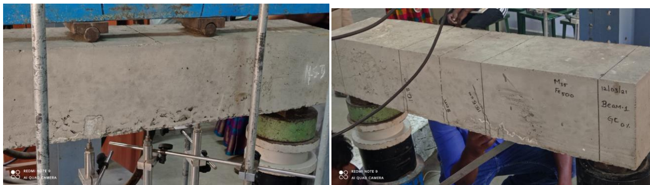
Fig 2– M I beam in test setup and failure mode
