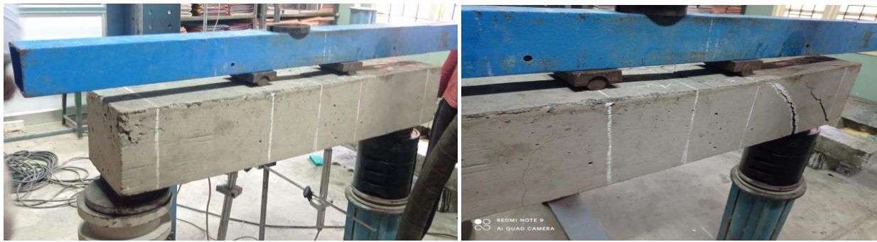
Fig 3- M I beam in test setup and failure mode
