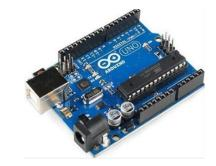
The Arduino Uno board is a microcontroller based on the ATmega328. It has 14 digital input/output pins in which 6 can be used as PWM outputs, a 16 MHz ceramic resonator, an ICSP header, a USB connection, 6 analog inputs, a power jack and a reset button
