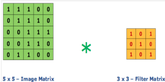
Figure 4: Image matrix multiplies kernel or channel grid
