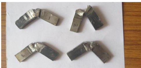
Fig. 5.23 Broken samples of MIG welding after impact test.
