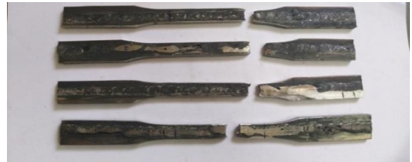
Fig. 5.12 Broken specimen welded by TIG welding after longitudinal tensile testing.
