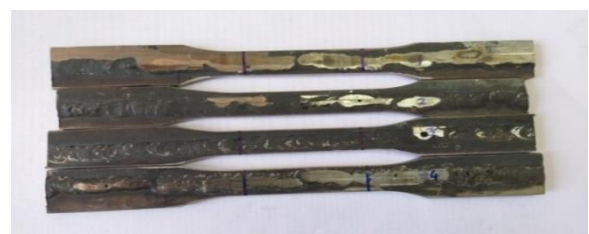
Fig. 5.5 Welded specimen using TIG welding for transverse tensile testing.
