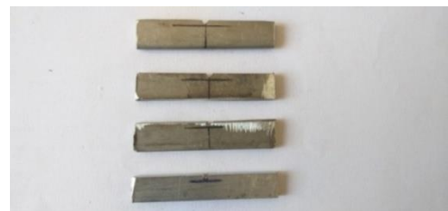
Fig. 5.17 ASS 304 base metal sample for impact test.
