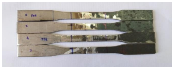
Fig. 5.5 Welded specimen using TIG welding for transverse tensile testing.
