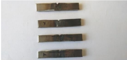
Fig. 5.20 TIG welded sample for impact test.
