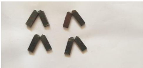
Fig. 5.22 Broken samples of mild steel base metal after impact test.
