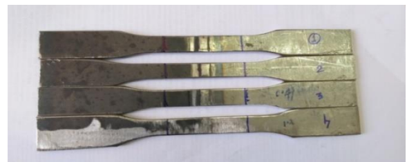
Fig. 5.3 Welded specimen using MIG welding for transverse tensile testing.
