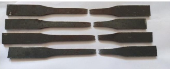
Fig. 5.8 Broken tensile test specimen of mild steel base metal in tensile test.
