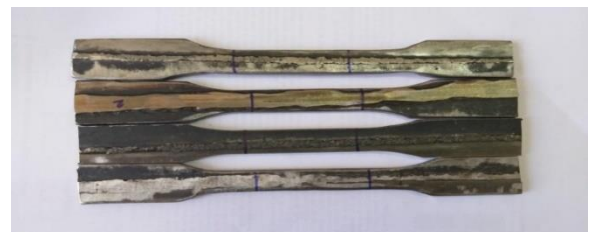
Fig. 5.4 Welded specimen using MIG welding for longitudinal tensile testing.
