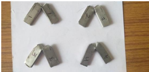
Fig. 5.21 Broken samples of ASS 304 base metal after impact test.
