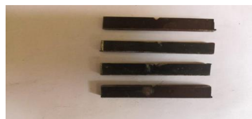
Fig. 5.18 Mild steel base metal sample for impact test.
