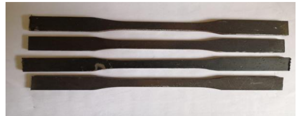
Fig. 5.2 Mild steel base metal tensile specimens.
