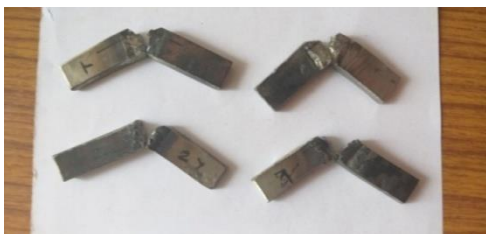
Fig. 5.23 Broken samples of MIG welding after impact test.
