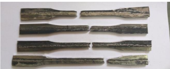
Fig. 5.10 Broken specimen welded by MIG welding after longitudinal tensile testing.
