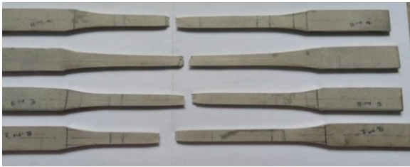
Fig. 5.7 Broken tensile test specimen of ASS 304 base metal in tensile test.
