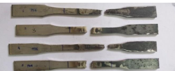
Fig. 5.11 Broken specimen welded by TIG welding after transverse tensile testing.
