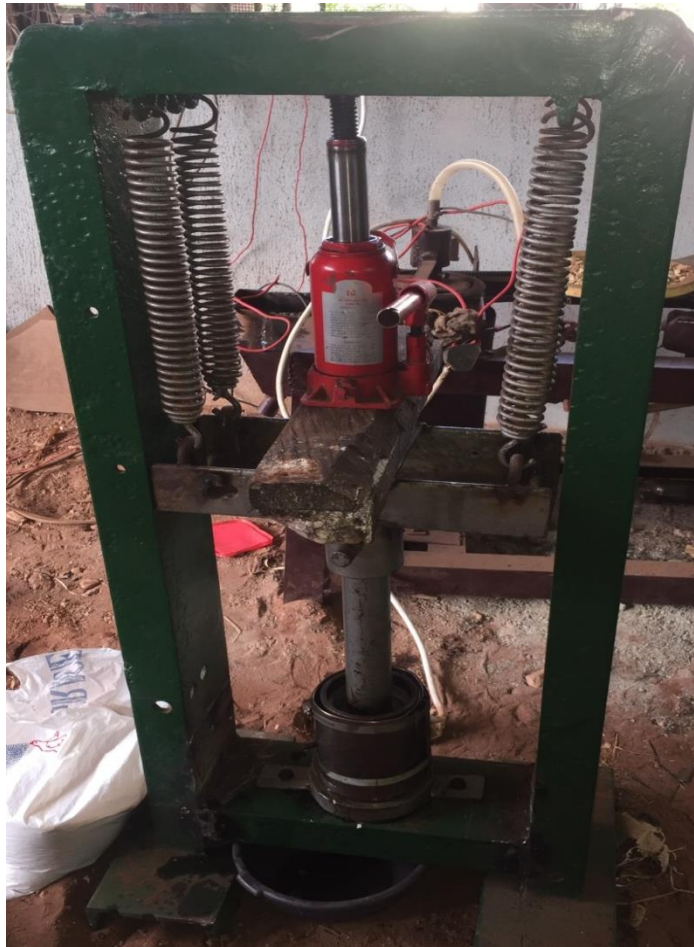
Figure 2: Pictorial view of the Hydraulic Press during Pressing Operation
