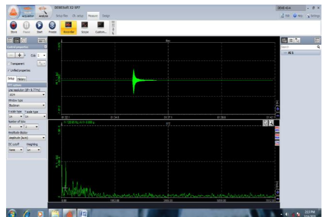
Fig. 5.4: FFT Test Results
