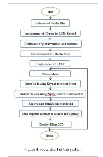
using Code Vision AVR IDE. Algorithm of the firmware depicted in figure 4. As per the requirement different menu assign for number and sequentially called. UART configured for transmitting and receiving the data. The Zigbee is configured in hoping mode, it is help full for long distance communication. The each Zigbee configured with different ID and share the data base station as well. All the functions and tasks are designed as per requirement and perform the allotted task sequentially.
