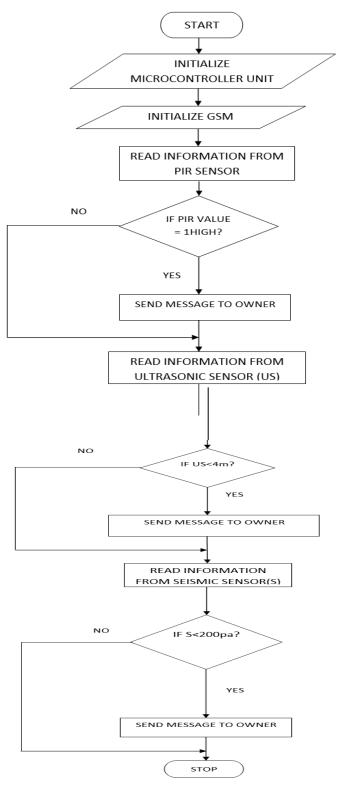
The Arduino Uno board and GSM are set up first. The values of the three PIR sensors are read and fed into the microcontroller. The system reads the ultrasonic sensor value when the PIR value is high or 1.
