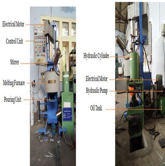
Fig -1: Stir casting machine
