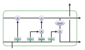
Forget Gate: the knowledge that not useful within the cell state is removed with the forget gate. Two inputs x\_t (input at the actual time) and h\_t-1 (previous cell output) are fed to the gate and multiplied with weight matrices followed by the addition of bias. The resultant is skilled an activation function which provides a binary output. If for a specific cell state the output is 0, the piece of data is forgotten and for the output 1, the knowledge is retained for the longer term use.
