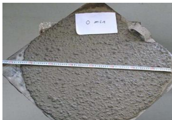
Fig3. Slump flow test
