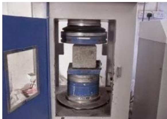
Fig5. Compressive strength test
