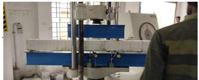
Fig .1. Testing set up for GFRC
