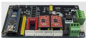
Fig.3.4 Assembled view of LBA-B-V4 CNC Shield with A4988 stepper motor driver.
