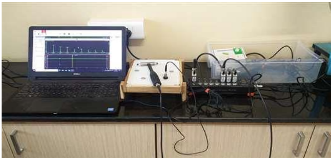
Fig. 8 Experimental Modal Analysis Setup
