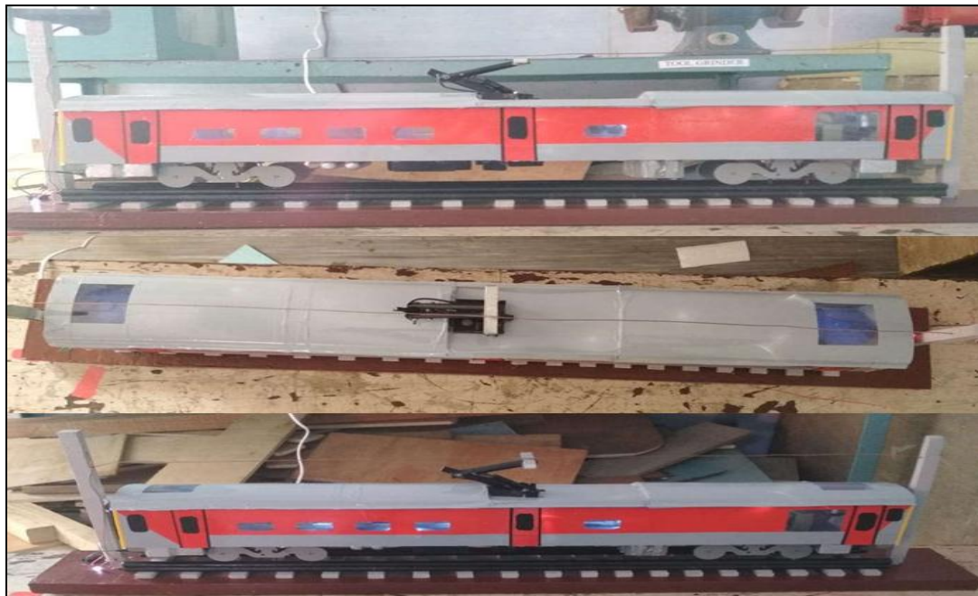
Photo-4: Proposed Prototype (Fabricated at RCF during training period) using Ratio-1:30 to the LHB coach
