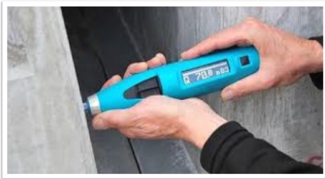
Figure 1-1 Schmidt Rebound Hammer Test
