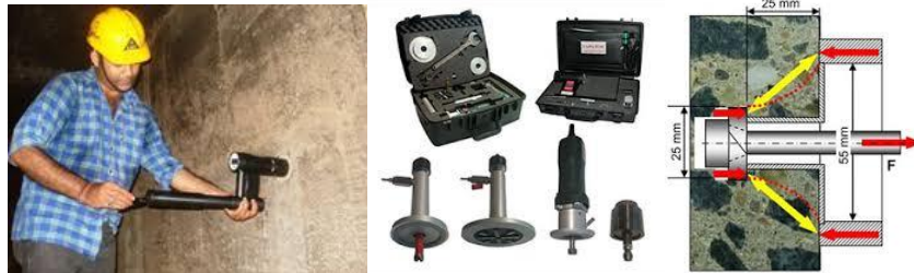
Figure 1-8 Cut and Pullout Test (Capo)
