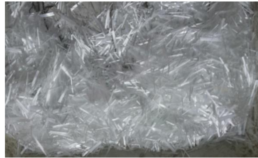
Fig 2: Cem-fil anti-crack alkaline resistant glass fibers
