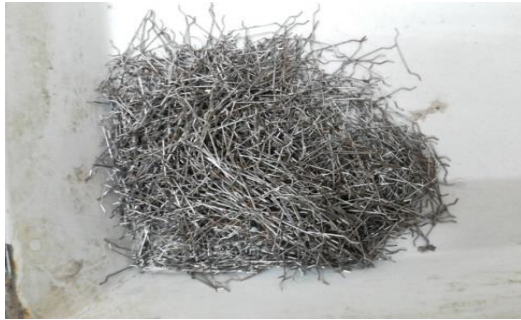
Fig 1: Hooked end steel fibers
